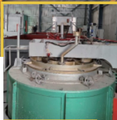
CARBURIZING FURNACE 渗碳炉
